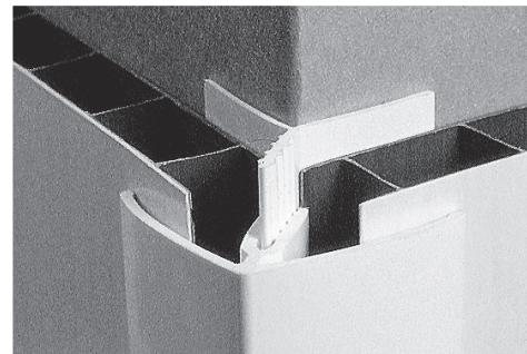
To form an external corner fix the mounting strip to the wall using wall plugs and flat head screws. Finish corner by clipping the front face into place.
