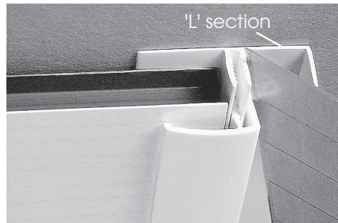
To start or finish a run of boards at a corner. Remove the 'L' section from the mounting strip using an appropriate knife.
