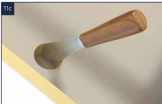
11c Remove remaining foam to back of plasterboard.
