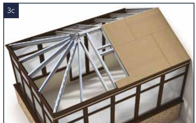
Continue fixing the plywood as per roof schedule.
