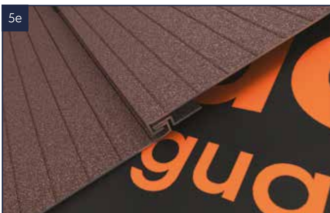
5e Hook nose of upper tile into lip of tile below ensuring a tight fit (the heel of your hand or a block of wood can be used to gently knock the tiles in tightly together).
