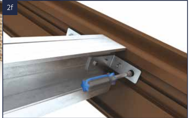
2f Ensure all roof sections are aligned to the pre-engineered positions and tighten into place. For Edwardian / Victorian hip cleats, tighten bolts on rafters first before tightening to ringbeam.
