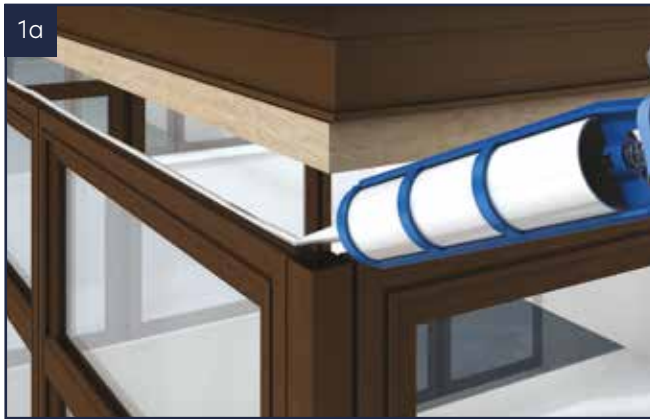
1a Silicone seal 70 x 60 mm timber packer to windows using low module silicone.
